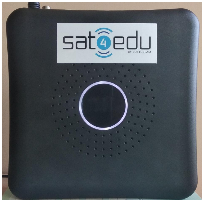
Figure 6. The display (LED ring) that indicates the state of the modem and connection
