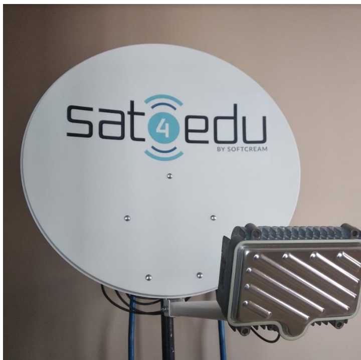
Figure 1. Satellite dish with signal converter
